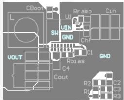
Figure 24. Recommended PCB Layout
