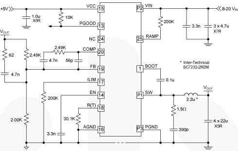
Figure 10. Application Circuit: 1.8Vout, 500KHz
