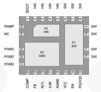
Figure 3. MLP 5x6mm Pin Configuration (Bottom View)
