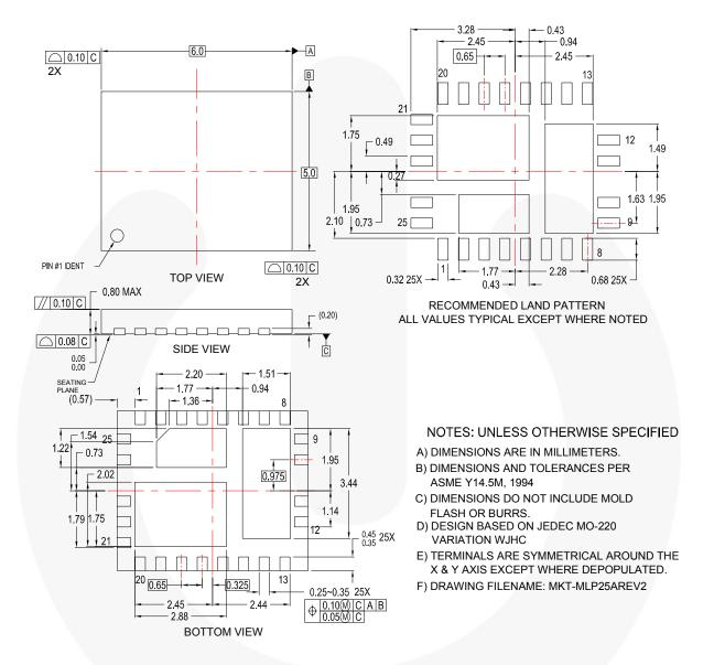
Figure 25. 5x6mm Molded Leadless Package (MLP)
