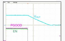
Figure 16. Startup with 1V Pre-Bias on Vout
