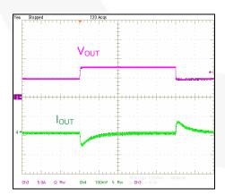
Figure 18. Restart on Fault
