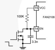
Figure 23. Enable Control with Latch Option
