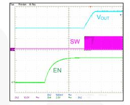
Figure 15. Startup, 3A Load
